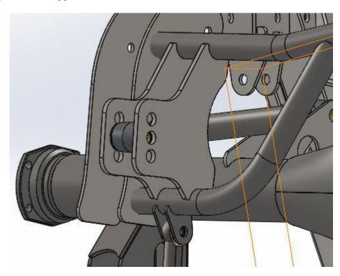
8) Time to install the axle brackets see measurements below. Be sure to tack weld them first and recheck measurements before fully welding all brackets. Tack the upper link mounts first. Then tack the left and right lower link axle brackets followed by the panhard bracket.
