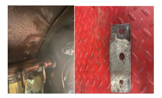
2) Next you will need to cut the upper link clearance holes. Please see attached pictures for measurements where to place them. The holes will be 4.5" wide and 5.5" tall. You will later use the supplied enclosures to seal these holes off from the elements.
