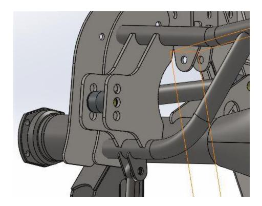
8) Time to install the axle brackets, see measurements below. Be sure to tack weld them first and recheck measurements before fully welding all brackets. Tack the upper link mounts first. Then tack the left and right lower link axle brackets followed by the panhard bracket that will locate against the driver side lower link mount
