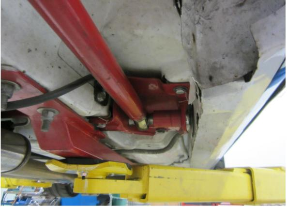
10) Once the links are installed install the panhard bar
