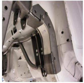
5) Install the left and right rear saddles. Make sure the saddles are flat on the frame rail and hold the saddles in place with a vise clamp / c-clamp. Drill the holes though the frame.
