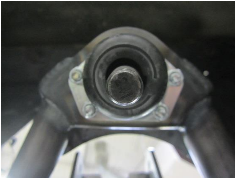
Upper Ball Joint Installed, Figure 20A
