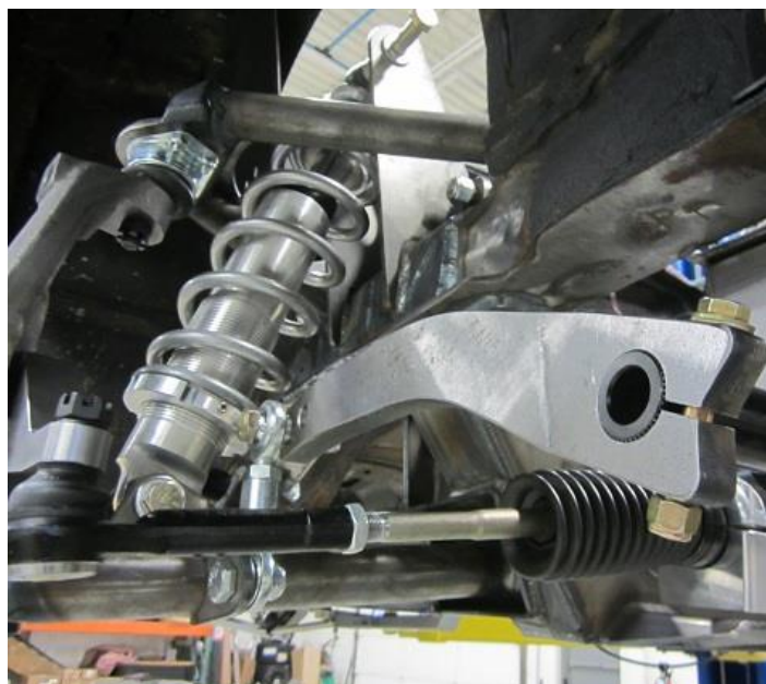
Splined Sway Bar, Passenger Side, Figure 38
