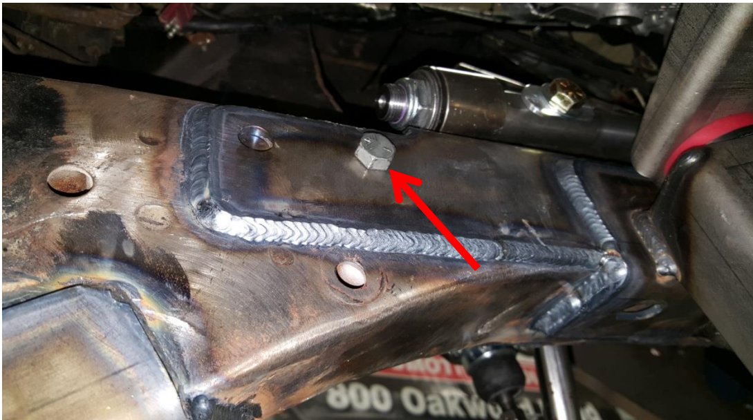
Slide Factory 7/16" Steering Gear Bolt though Saddle and Factory Frame Rail, Figure 8
