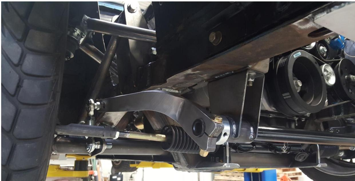
**PASSENGER SIDE ARM, LOCK COLLAR AND BUSHING, FIG. 9**
