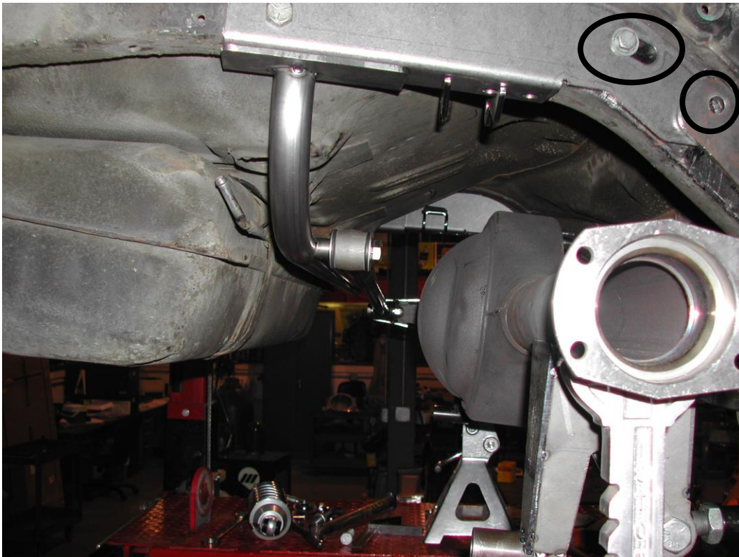
Figure 2. Passenger side frame rail brackets, note bolt location in top of slots (circled)
