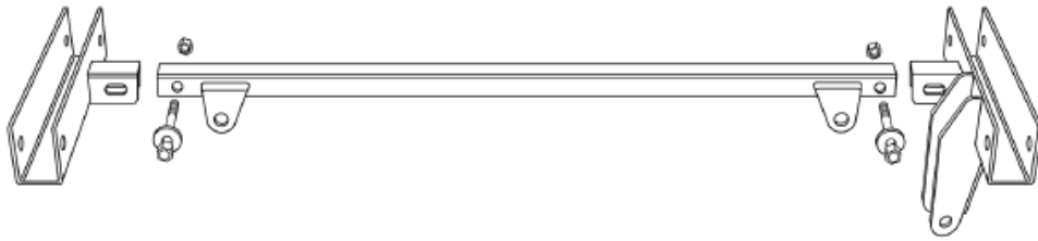
Figure 1- Top Crossmember Assembly
