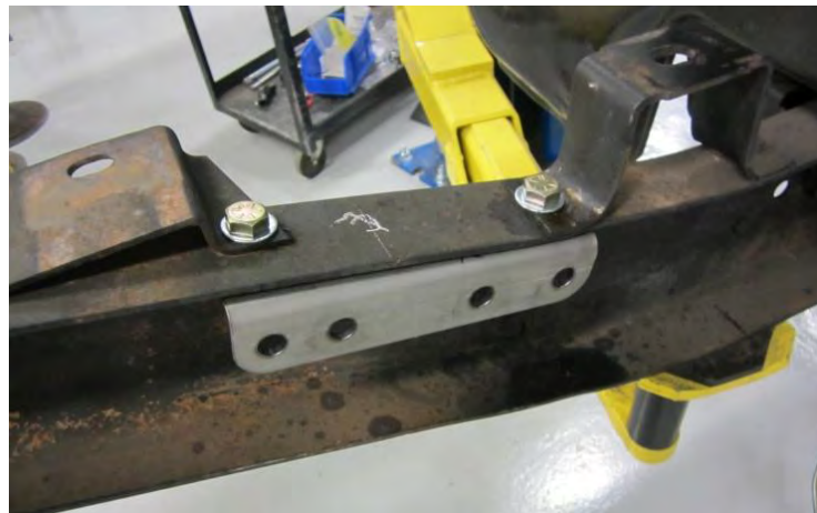
View of Drivers Side Frame Rail, Bracket Installed Figure 3
