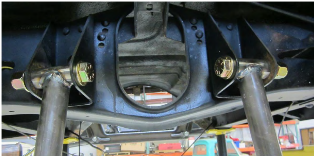
Installing Reinforcement Links In Factory Truck Arm Mounts
