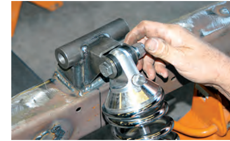
14) Bolting the coilover shock to the upper tower started the installation. At this point the bolt was finger-tight just in case it would have to be removed.
