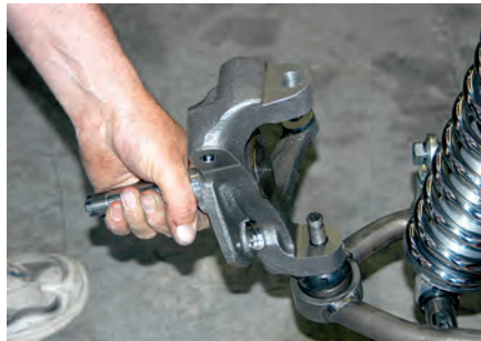
17) The spindle was connected to the lower A-arm. The lower ball joint is long, so spacers are used to make sure the castle nut aligns with the cotter keyhole.
