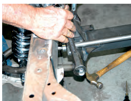
24) The lower A-arm bolt and Nylok locknut was secured with a pair of 15/16-inch wrenches.
