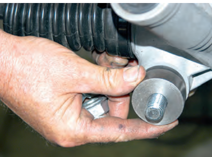
25) Before the rack-and-pinion can be installed, you have to install the bolts with a pair of spacers and washers.
