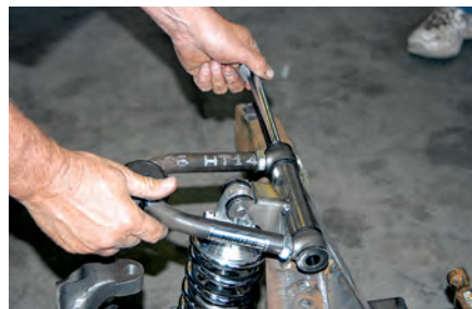
18) Using the other long bolt supplied in the kit, the upper A-arm was installed. This connection also uses the large washers supplied in the kit. The upper bolt is secured with a Nylok locknut.
