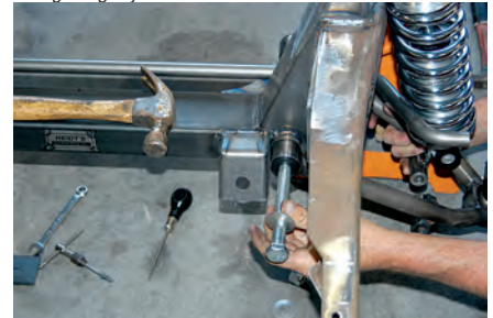
15) The lower A-arm was installed using the long bolt supplied in the kit. Washers are supplied to rest against the urethane bushings.
