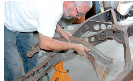
3) The crossmember was easy to remove when it was moved back to the wider part of the frame. Since these crossmembers are worth money to nostalgia rodders, owner Bob O'Bryant wanted to keep it in good condition. The radiator mounts are still attached to the crossmember and will have to be removed and used after the new front suspension is installed.
