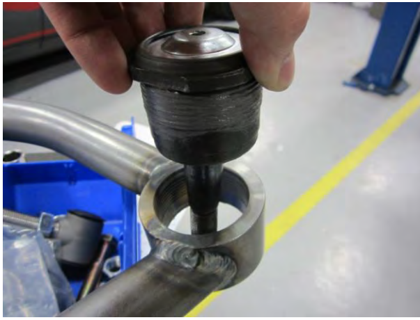
Installing Ball Joint
