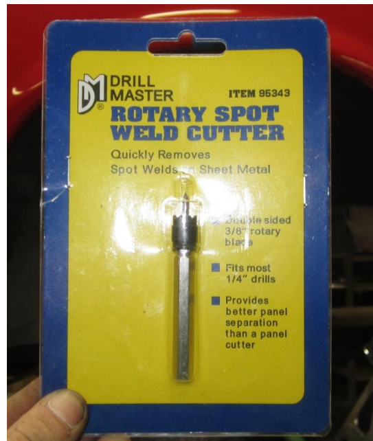
Rotary Spot Weld Bit, Figure 1
