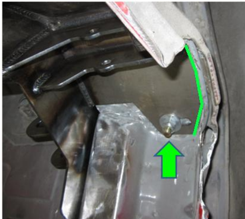
Trim Saddle at Green Line for Custom Fitment, Fig. 20
