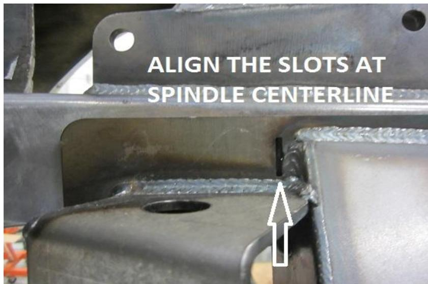
**K-Member, Vertical Slot is the "Spindle Centerline", FIG. 1**
