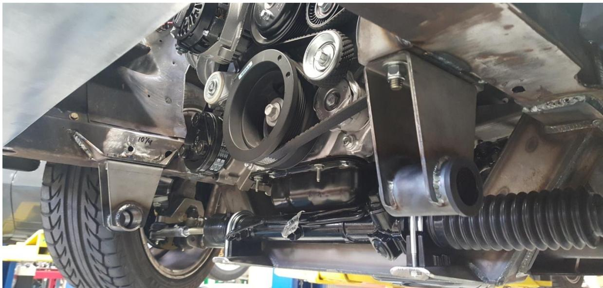
**Drop Down Mounts, Poly-Bushing Positioned on Outside, FIG. 4**
