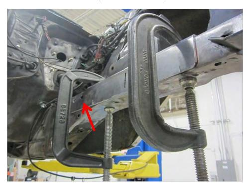
Slide Factory 7/16" Steering Gear Bolt though Saddle and Factory Frame Rail, Figure 8
