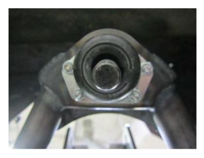
**Upper Ball Joint Installed, Figure 20A**
