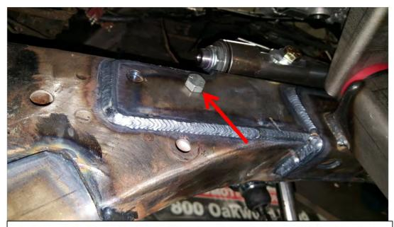
Use OEM 7/16" Dia. Steering Gear bolt, in Front Hole of Shock Tower Mount. Mounts in factory frame hole.
