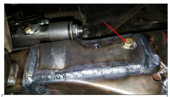
Use OEM 3/8" Dia. Idler Arm Bolt, in Rear Hole of Shock Tower Mount to locate. Mounts in Factory Frame Hole.
