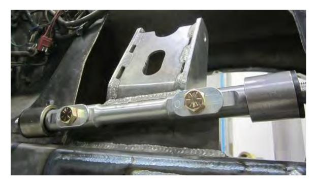
Fully Assemble Upper Control Arm with 0" Control Arm Slugs, Figure 21D
