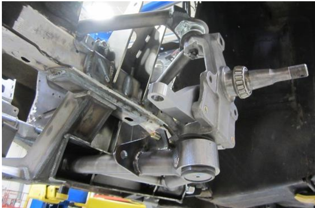
Driver Side, Spindle attached to Ball Joints, Figure 25
