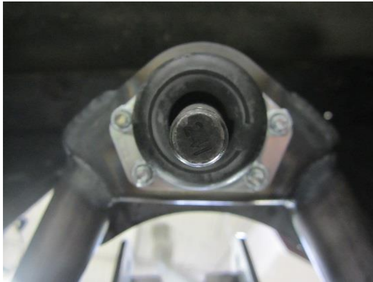
Upper Ball Joint Installed, Figure 20A
