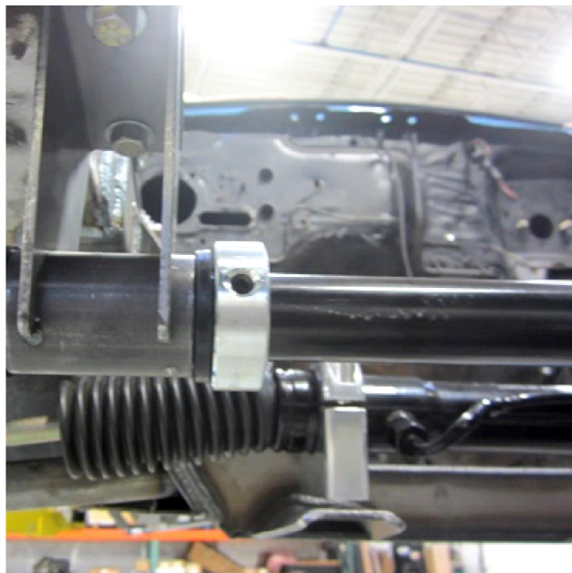
Bushing & Clamping Collar from Inside of Sway Bar Mount, Passenger Side Shown, Figure 37
