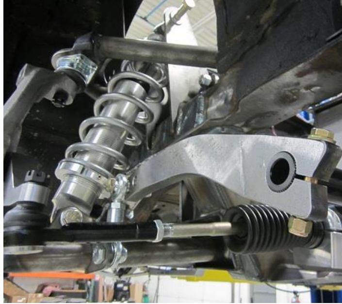
Splined Sway Bar, Passenger Side, Figure 38
