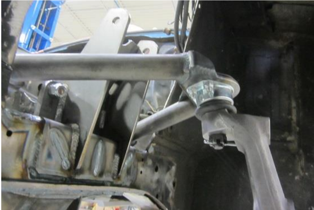
Upper Ball Joint Castle Nut installed, Figure 26
