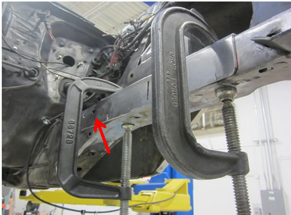
Slide Factory 7/16" Steering Gear Bolt through Saddle and Factory Frame Rail, Figure 8
