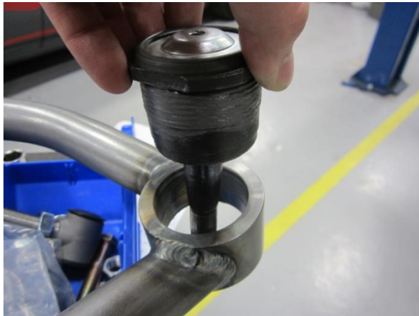
Installing Ball Joint
