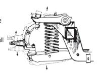
Correct design results in correct camber action - and no bumpsteer
