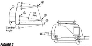
Now we have added the stock Mustang II steering rack in the stock Mustang II location using the stock Mustang II tie rod ends. Notice the radius of the rod ends (2) matches the radius of the spindle. Also, more importantly, see that the inner tie rod pivot (3) is IN LINE with the inner pivots (4) & (5) of the upper and lower arms. This is absolutely necessary. Ford Motor Co. did their homework.
