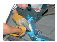
10) After all of the measurements were made and the crossmember was located correctly, it was tack-welded to the frame.
