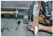
**15)** The lower A-arm was installed using the long bolt supplied in the kit. Washers are supplied to rest against the urethane bushings.
