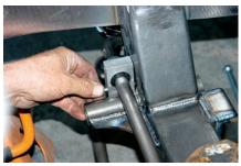
13) The Swaybar block was bolted to the crossmember on the bottom, and when it was in place, the upper bolt hole was drilled and tapped. Doing it this way ensures that the bolt holes will line up perfectly.
