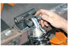
14) Bolting the coilover shock to the upper tower started the installation. At this point the bolt was finger-tight just in case it would have to be removed.
