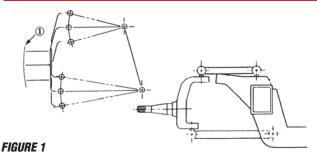
This is a correct Mustang II front suspension in a street rod, when the stock Mustang II suspension locations are used. Notice the parallel upper and lower arms. Also notice there is minimal camber change and almost flat radius (1) in the movement or the spindle during suspension travel.
