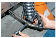
16) The coilover shock was connected to the lower A-arm. This is a long bolt because it is also used to secure the Swaybar connector. The bolt is installed from the front and O'Bryant made sure the Swaybar connector was installed first.
